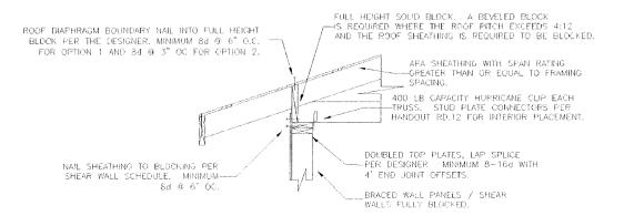
OPTIONS 3 & 4: THESE CONFIGURATION MAY BE USED IN LIEU OF FUEL HEIGHT BLOCKS ABOVE EXTERIOR WALLS FOR TRUSSES WITH HEELS OF 11 1/4".
